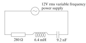
(i) Use a phasor diagram to show that the impedance of an LCR circuit is given by
